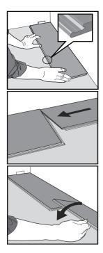
Figure 1. *First plank, first row.* Tongue side against the wall, groove side facing out. Later, after the third row is installed, you can easily position the flooring against the front wall with a distance of approximately 3/4".
