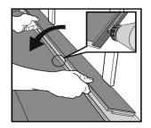
Cut off the locking element with a chisel and use floating floor adhesive on the adjusted strip; push the planks horizontally together.
