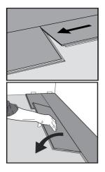
Figure 7. General; distances between short ends. Minimum distance between short ends of planks in parallel rows should be 12".
